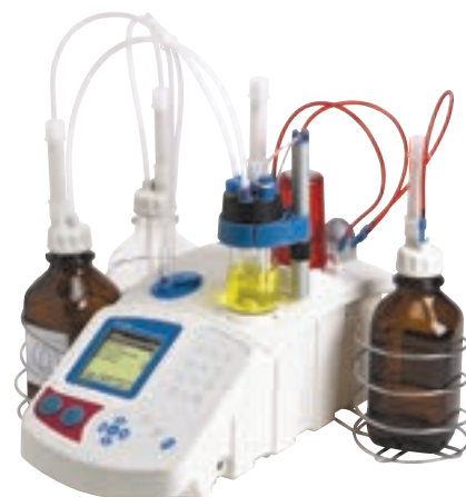
Volumetric Karl Fischer for quick moisture content determination between 0.1% & 100%
