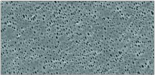
Polyamide Membrane (Type NL 17, 0.45 μm) Electronic Micrograph (Magnification 1000x)
