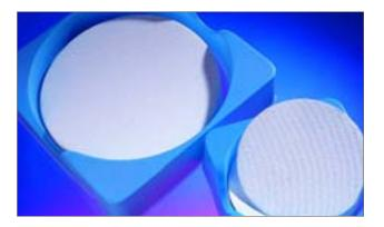
These acid treated low metal filters are available in 47 mm, 90 mm, 110 mm, 125 mm, 142 mm and 150 mm diameters. The 90 mm filter is required for volatile samples and use with a Zero Headspace Extractor. The 142 mm filter is typically used with non-volatile samples in an approved jar.
