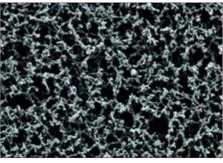
Cellulose Acetate Membrane (Type ST 68, 0.8 µm)
