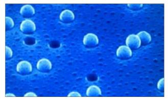
Electron Micrograph of Cyclopore Membrane
