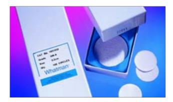
Whatman EPM 2000 was selected by the EPA to be the standard filter for use in the nationwide network of HiVol air samplers. Sheets are individually numbered to facilitate identification.
